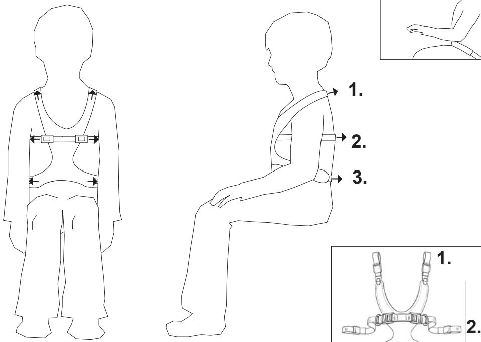
Use the fittings (A) and (B) on the chair to mount the sternum belt. If no fittings are mounted, please use the enclosed fix locks and belt fittings to mount the sternum belt as shown on picture (C) and (D). Any doubt on mounting, please contact a local therapist or authorized R82 personnel.
