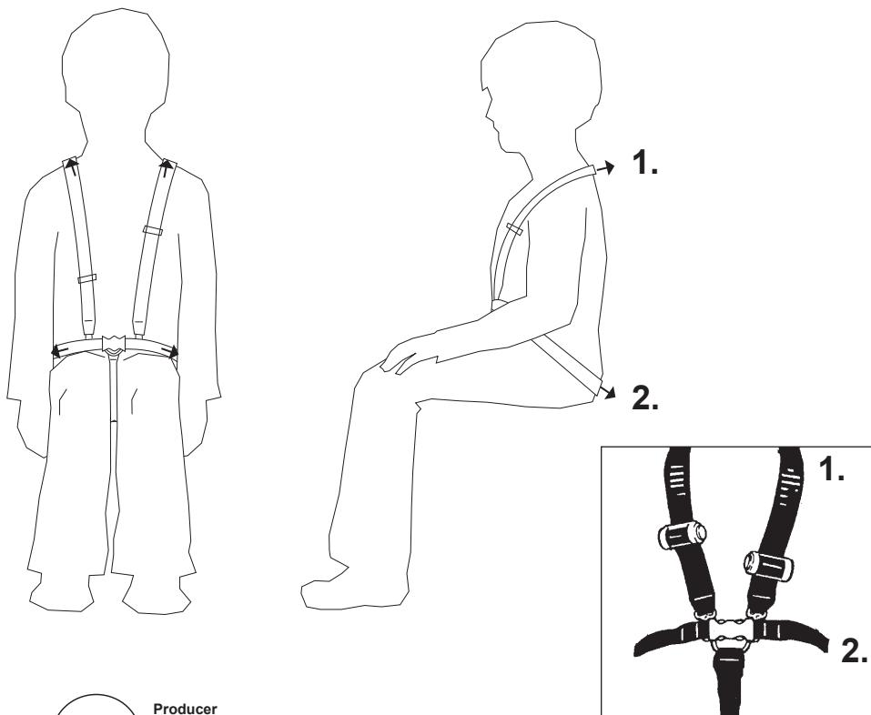
Use the fittings (A) and (B) on the chair to mount the 5-point belt. If no fittings are mounted, please use the enclosed fix locks and belt fittings to mount the 5-point belt as shown on picture (C) and (D). Any doubt on mounting, please contact a local therapist or authorized R82 dealer.
