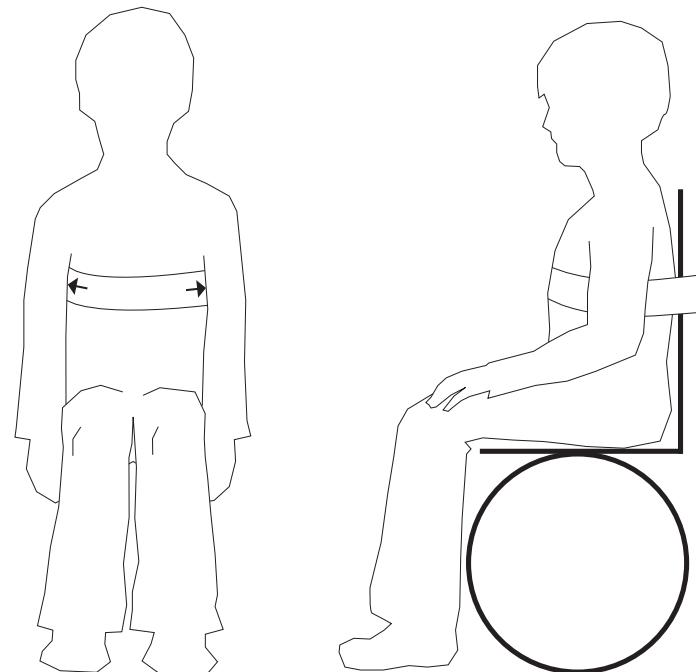
The belt goes around the persons chest and around the back of the chair. Use the velcro for closing the belt and lock with the metal lock. Any doubt on mounting, please contact a local therapist or authorized R82 personnel.
